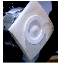
Above, Underside of lid showing chucking recess with finished convex design.
