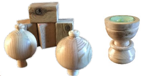
Gary Woodhouse has joined some waste blocks to turn two sphere finials for a quilt hanging pole. He has also made a tealight holder with a captive ring.
