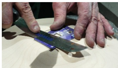
Above protecting the work with a card. Left Ben's finished platter showing colour and pimples. The natural wood is the area that was masked off. Right More colouring ideas.
