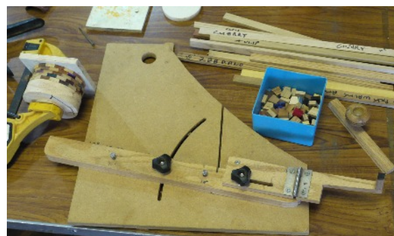
Ben's worktable showing assorted segments, sled with adjustable angle guide and hinged sliding dovetail stop. Note also prepared rings glued and clamped.
