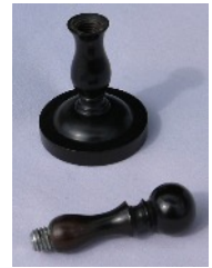
A two part chess piece joined with a threaded insert. Made by Mike Knight.
