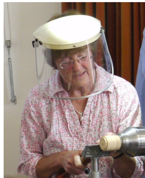
Maggie Wright demonstrating thread chasing
