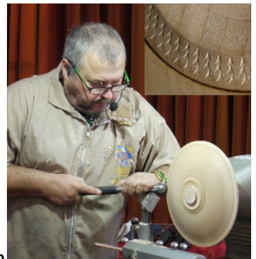
Mick Hanbury using the texturing tool. Inset showing design created. Below. Wooden hairdryer holder fitted over tool post
