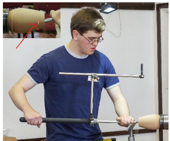
Fred Mitchell hollowing with the laser guide attachment. Inset top left shows the laser beam on the work nearing the required depth.
