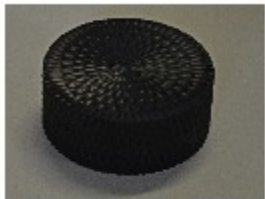
An example of Maggie's ornamental turning. A threaded patterned box in African Blackwood.
