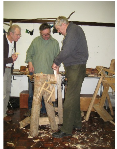
Neale Sands having a go at riving the feathers. Notice Sean's leg vice and shaving brake.
