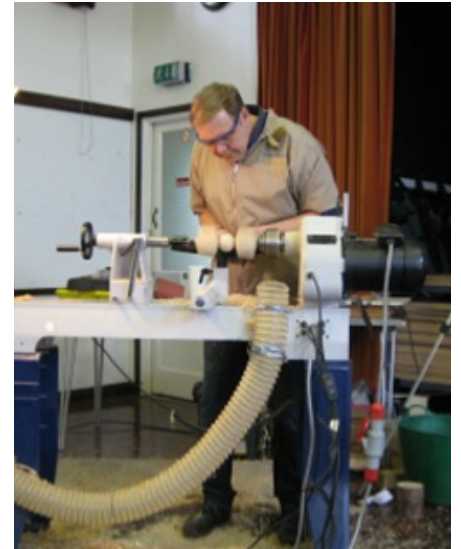
Simon turning an off centre candlestick
