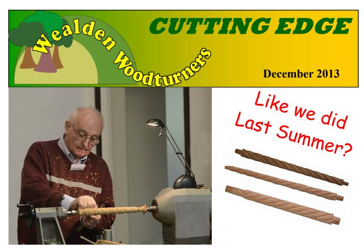
**Last month** we took a trip down memory lane with Mike telling us about his experience of making barley twists by the hundred for clock cases, each requiring four twists. After explaining the marking-out process Mike produced twists of different designs with the aid of a few simple hand tools. Each had to be offered up to its counterpart so as to ensure there were a matching pair.
